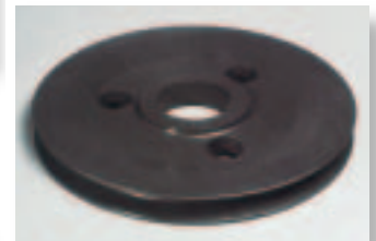
Picture 3 - This 19" diameter Nylatron® GSM PA6 sheave requires only finish machining of the bore for bearing press fit.
