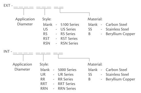
Example: EXT 050 US - External Spiral Retaining Ring, 0.500" Application Diameter, US Series, Carbon Steel
