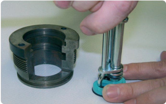
3. Rod seal properly folded for ease of installation
