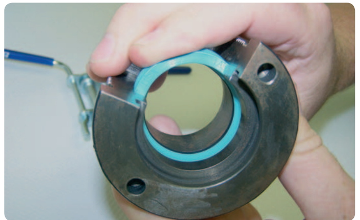
6. Rod seal properly installed
