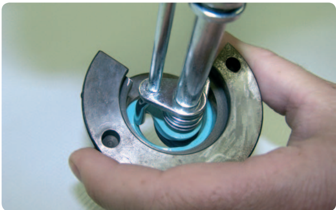
5. Tool positioning rod seal in the groove
