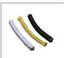
**Braided Packing** - Hi-Tech Seals stocks braided packing made from Aramid, PTFE, Graphite, GFO®, and Grafoil®. Typical applications include rings for pumps, mixers, valve stems, tank lid seals, and manway gaskets. Specially designed packing with braided stainless steel or inconel wire for added reinforcement in high pressure applications and silicone core packing for added resilience are also available.
