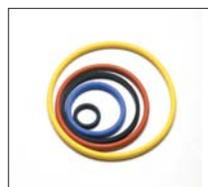
**O-Rings** - Hi-Tech Seals offers a wide variety of materials and durometers in one of the largest inventories in North America for O-Rings, X-Rings, and Square Cut Rings. Whether for high or low temperatures, caustic environments, abrasive wear, or high pressures, Hi-Tech Seals can deliver. Common materials include: Nitrile, Viton®, HNBR, Aflas™, EPDM, Neoprene, Perfluoroelastomer, and Urethane. O-Rings are available in imperial and metric sizes.
