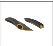
**Extruded Profiles** - Hi-Tech Seals offers extruded profiles in continuous lengths of material that can be cut, formed to shape, and bonded together by gluing or vulcanizing the joint. They make an excellent low cost seal for keeping out air, dirt, and moisture.
