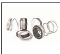
**Mechanical Seals** - Hi-Tech Seals stocks rubber bellow mechanical seals for pumps and mixers. Face materials include carbon, ceramic, ni-resist, tungsten, and silicone carbide for a wide variety of applications.
