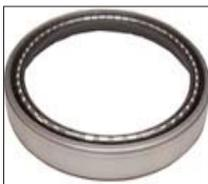
**Large Bore Rotating Shaft Seals** - Hi-Tech Seals offers a complete line of large bore, heavy duty oil seals. These seals are specifically designed for shaft sizes over 5 inches in diameter with high rotational speeds, heavy torque, or misalignment. Our L2M shaft seal has reinforced steel walls and a finger garter spring combination for keeping the seal tight in the most demanding applications.
