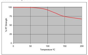
**Heat Aging**Aged at temperature indicated - Tested at (22°C).
