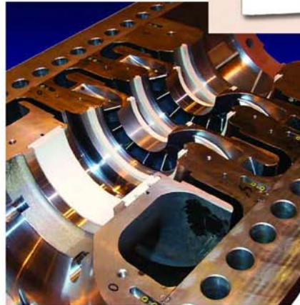
Cross-section of horizontally split high-performance process compressor utilizing polymer labyrinth seals. Photograph courtesy of Elliott-Company Div. of Ebara Corporation.
